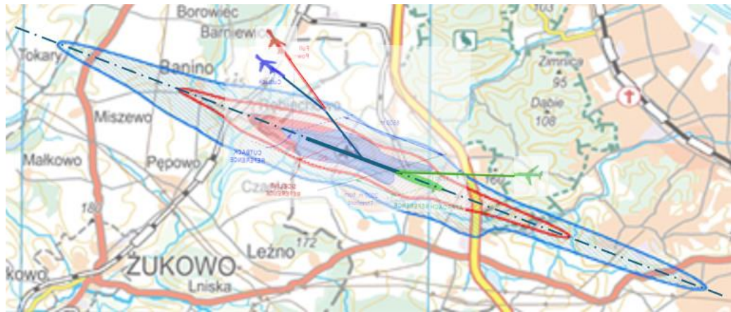
Fig. 6. Modular approach to evaluation of noise, fuel burn and engine emission metrics by ADFPP: combined example for AN exposure assessment is shown by comparison of noise certification, footprint (both shown in Fig. 4) and airport scenario (Fig. 2) platforms (Source: Authors’ own work)
