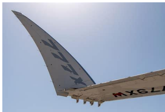
Fig. 2. Boeing 777X Folding Wingtip Technology Enhancing Compatibility with Existing Airport Infrastructure (Boon & Pande, 2023)
