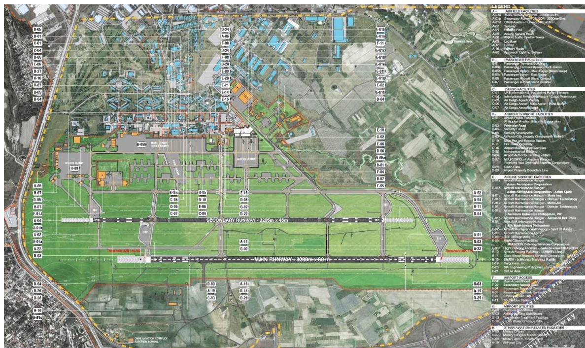
Fig. 4. Layout map of Clark International Airport highlighting the main runway, taxiways, terminals, and apron configurations' compatibility with wide-body aircraft such as the Boeing 777X (BCDA & IFC, 2018)
