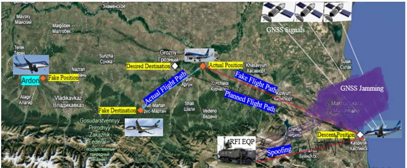
Fig. 5. RFI activation result on the aircraft flight J2 8243 trajectory paths (need to place on horizontal layout) (Source: Author’s own work)
