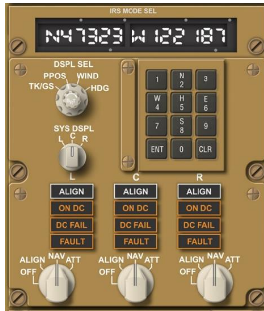
Fig. 7. A typical IRS control panel and display unit used on Boeing 757/767 (Flightvectors, 2025)
